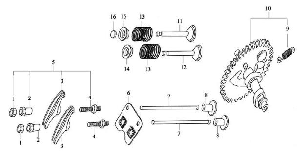
Note: When ordering parts from this list, specify: **Parts List E**, CAMSHAFT AND ROCKER VALVE ASSEMBLY and the ITEM No.
